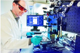
Image of the current maskless laser lithography setup at Joanneum Research MATERIALS
